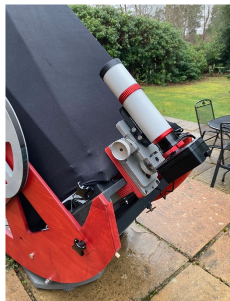
The eFinder integrated with ScopeDog on my telescope
