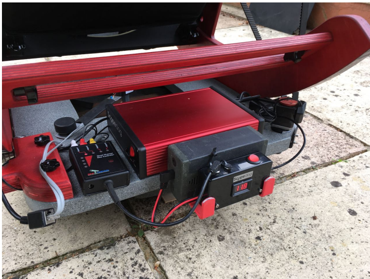
ScopeDog and accessories mounted on my telescope base
