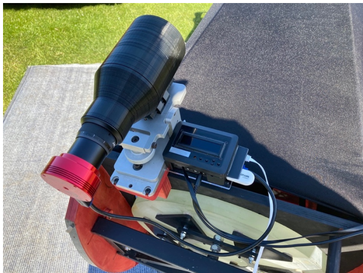
Figure 3 - The author's 'eFinder' The adjustable mount isn't now required
