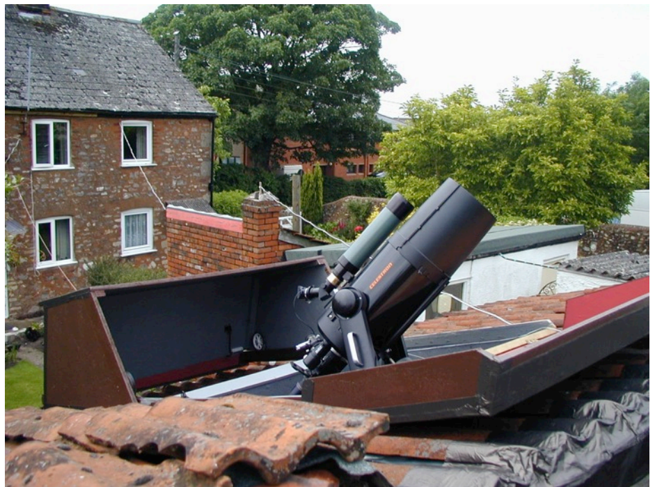
Despite a number of fairly close buildings and trees, a good coverage of the sky is seen from the top of the outhouse roof. The roll-off roof can be pulled towards the telescope to shield the observer from stray lights. This view is approximately due North. Photograph Keith Venables.
