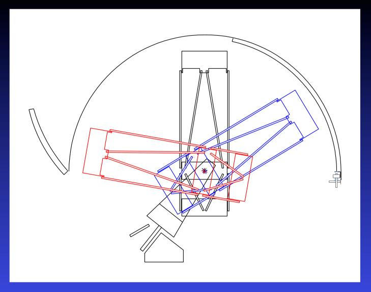
A 3.2m (11ft) dome would be required, mounted at least 1m above the telescope base.
